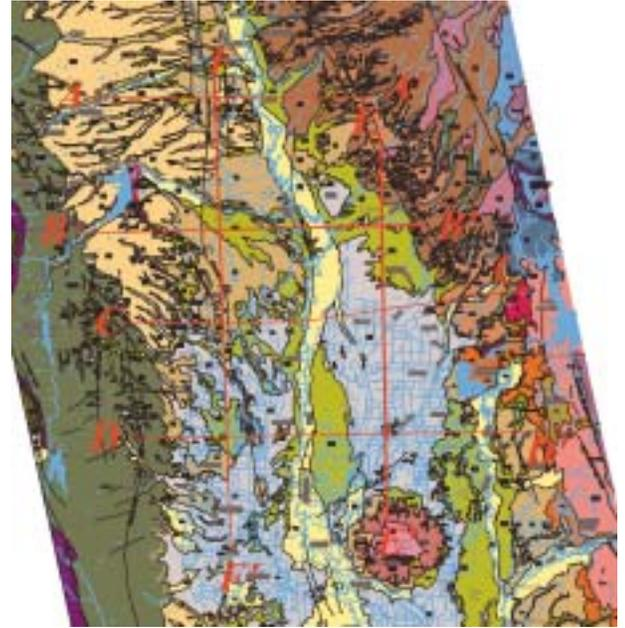
**Figure 1.** Northern Sacramento Valley Geologic Map. Red lines illustrate geologic cross-sections used in investigations of the northern Sacramento Valley aquifer systems since 1997. The legend of corresponding geologic map units and names is below.
