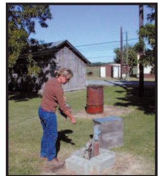
Figure 2. Measuring the depth to water table through an entry point in a domestic well with a metal tape.
