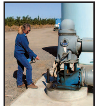
Figure 3. Measuring the depth of water table in an irrigation well with an electric sounder. Note pipe provides entry into well casing.
